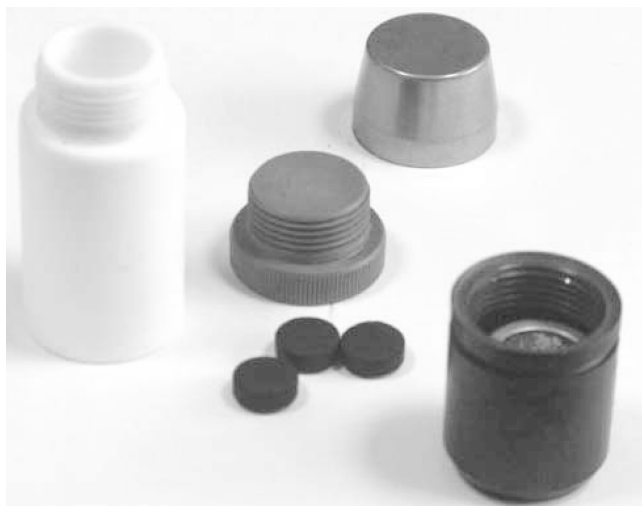
Figure 2 Set of LS vial, charcoal canister, and charcoal tablets
